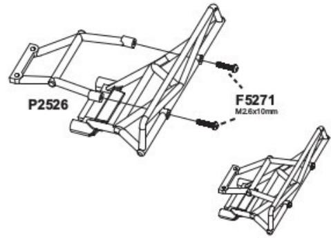
**Short Course Truck Chassis System Assembly View 底盘系统装配图**
