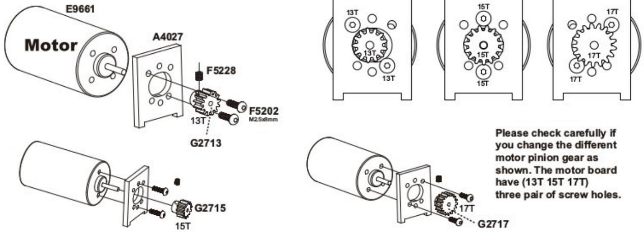
Monster Truck Chassis System Assembly View 底盘系统装配图
